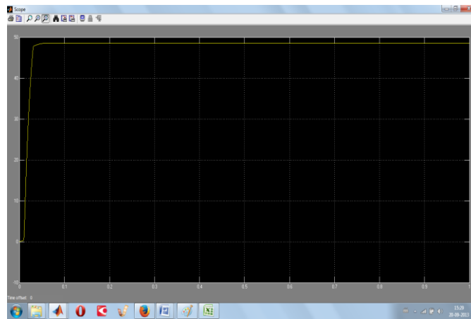
Fig.16 Boost Operation (Buck-Boost) (24 V to 48 V)
